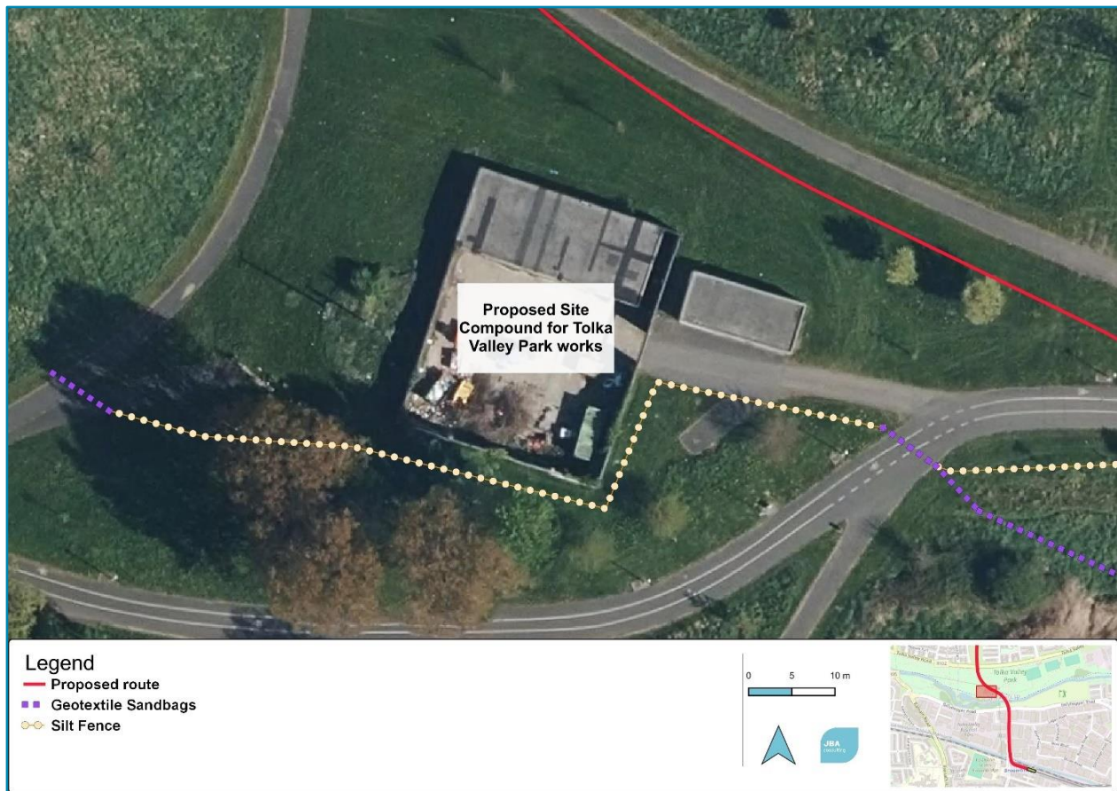
Figure 7-5: Indicative installation locations of silt fences and geotextile sandbag barriers (Tolka Valley Park) (Bluesky, 2024)
